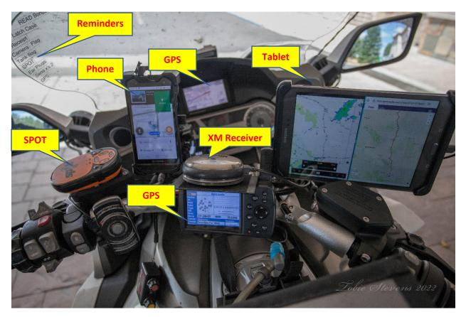
All riders have some tracking means, the Vooks use a Spot device. This communicates via satellite, so no worries about cell phone reception in the boonies. The XM Receiver is likely gathering weather radar which will display on that ancient GPS it's mounted on top of. Reminders or other notes on the windscreen can be super helpful during a ride like this. As an example here, the Spot tracker times out and a reminder to ensure you are still tracking can avoid disappointment later.
